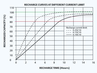
This means it will recharge the same battery approximately 1.4 times faster than a UPS with 3kW of charging power, or alternatively 2 times faster than UPS with 2kW of charging power. It can charge a battery of 1.4 to 2 times larger capacity (Ah) in the same amount of time.
